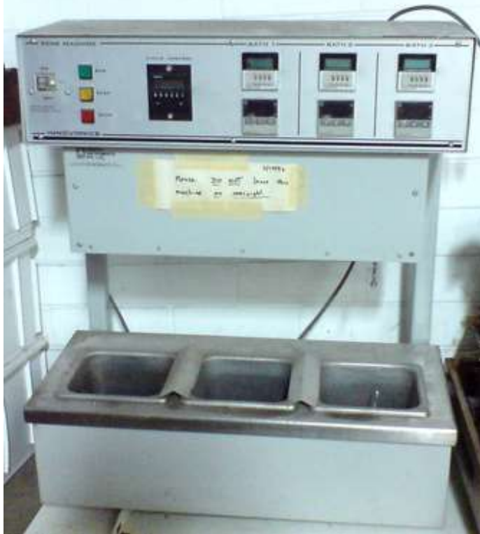
An older, three-temperature thermal cycler for PCR
