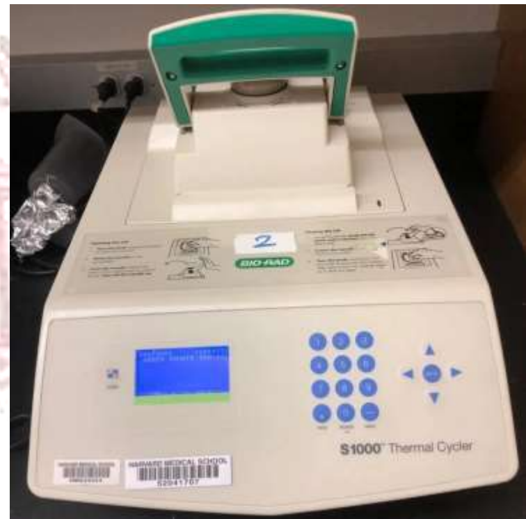
A 96-well plate modern thermal cycler for PCR
